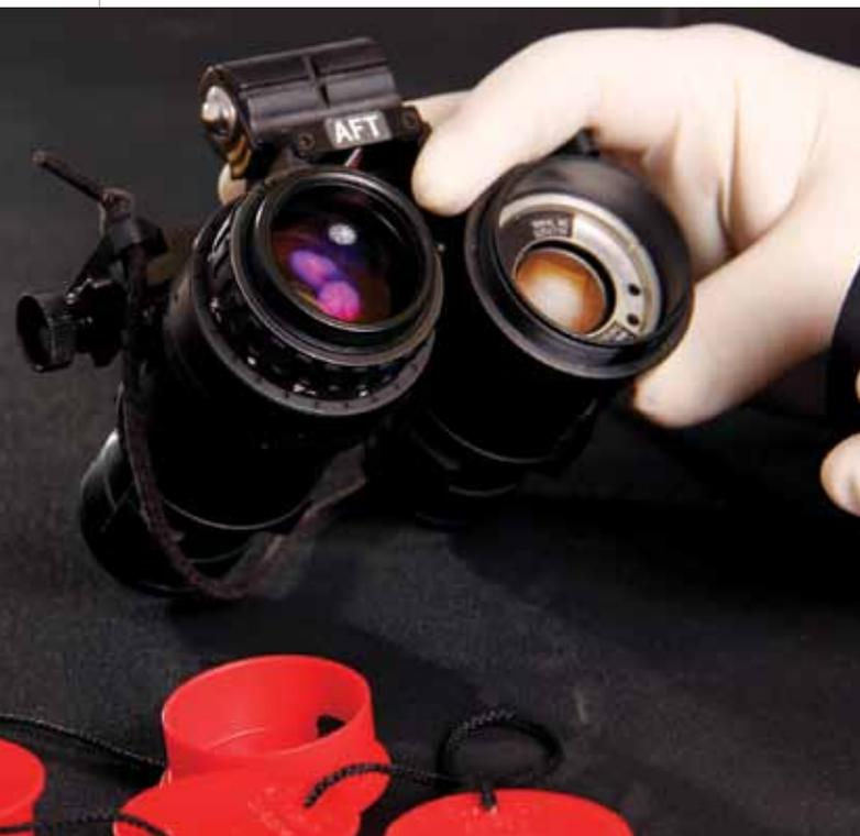
NVG Lens Assembly, Courtesy of Night Flight Concepts
